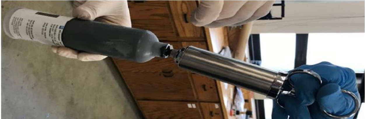
FIGURE 36. Air injecting into the sealant material before performing the experiment.
