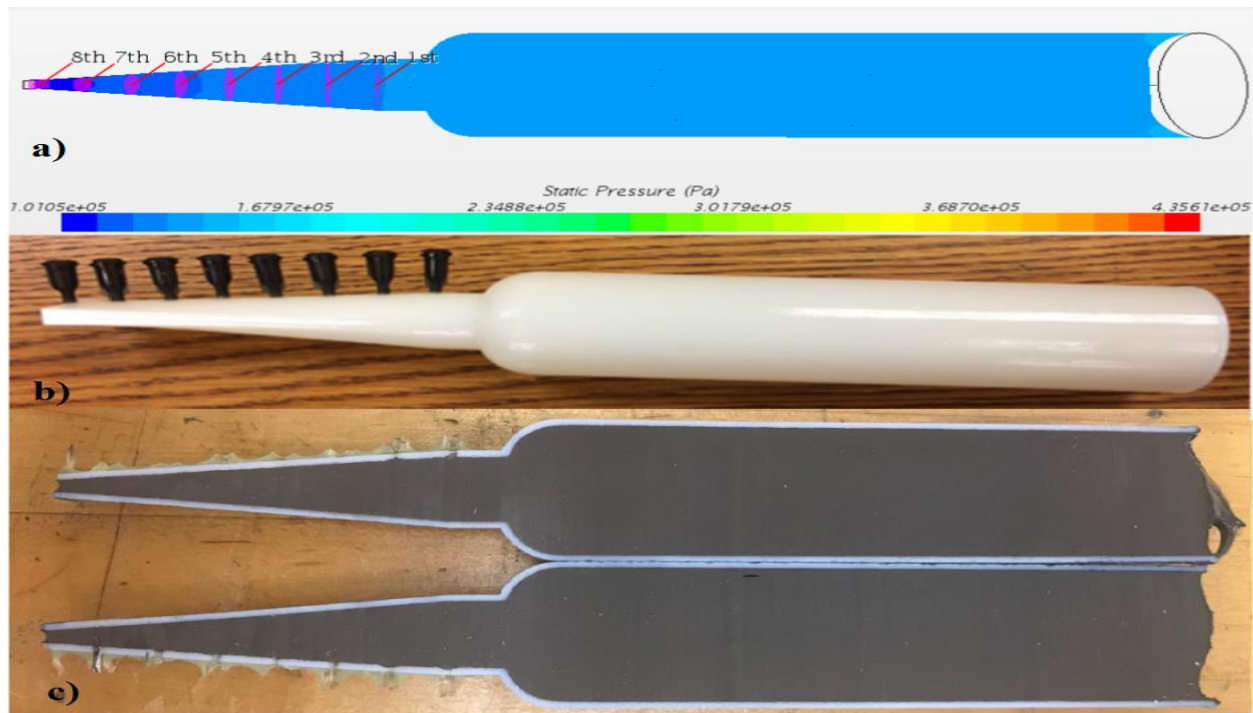
FIGURE 39. a) Sections in simulation software, b) sections in printed module, c) sections in sliced cure sealant inside the module.
